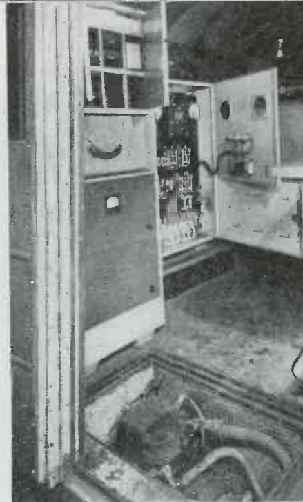
This close-up view was made through the windshield and shows arrangement of the two RCA recording lathes, with the operator in normal position seated at the console controls. Right, below, is a view showing the insulated well holding the 1 kw motor-generator set
