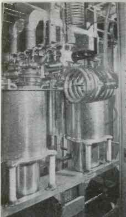
Fig. 5 (Left)—Massive construction of the 100 KW International broadcast transmitter, KGEX. Fig. 6 (Above)—The exciter cubicle of the transmitter showing first and second PA stages
