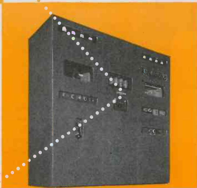
Collins 231D-13 —Nominal power output: 3000 watts phone; 5000 watts CW. Frequency range: 2 to 18 mc. Ten quick-shift frequencies.
