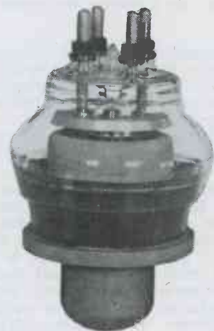
Fig. 4—The GE Type GL-880 Tube which made possible high power at high frequencies
