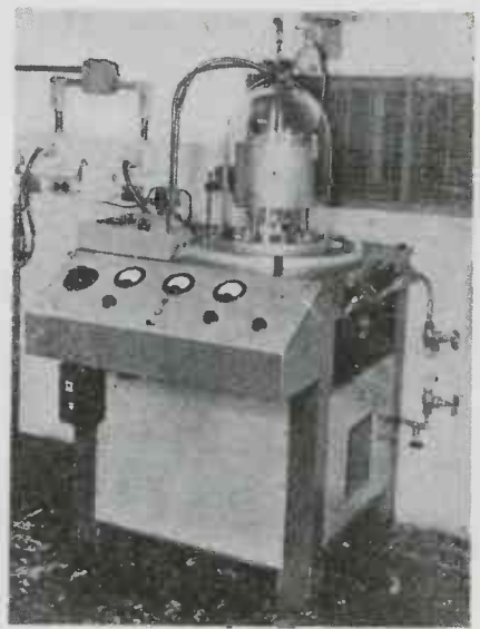
Complete set-up for evaporating monomolecular coatings onto lenses, using electronic vacuum gage and photoelectric determination of spectral reflection minima
