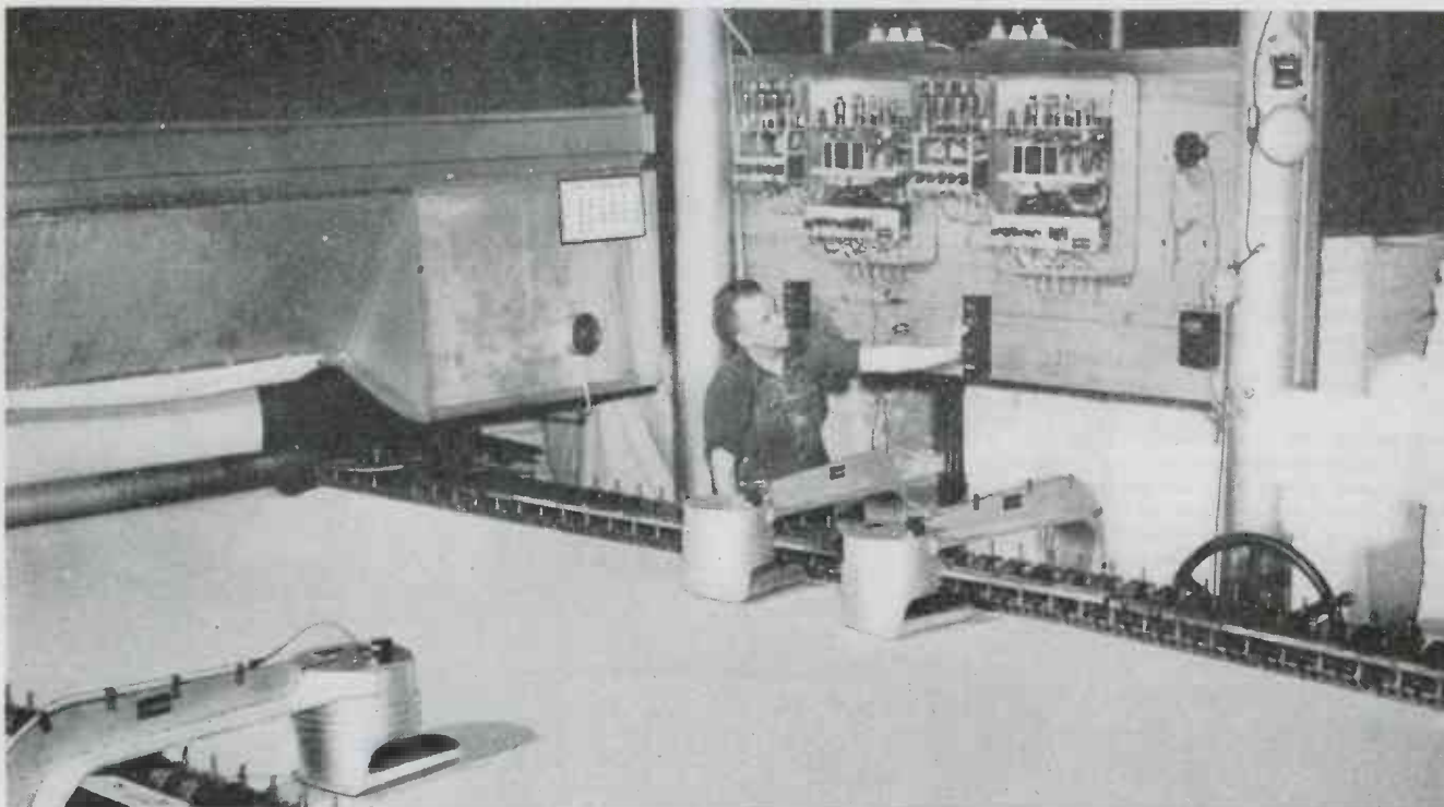
Electronic control equipment for weft straightening as used in the textile industries. The main control is in the background with operator ready to start the mechanism manually. Tenter, with scanning mechanism in place appears in the foreground
