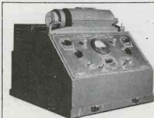
Above, Signal Corps Radio telephoto transmitted from Italy. Caption is part of picture, which is transmitted in seven minutes. Left, front view of new model Acme telephoto transceiver
