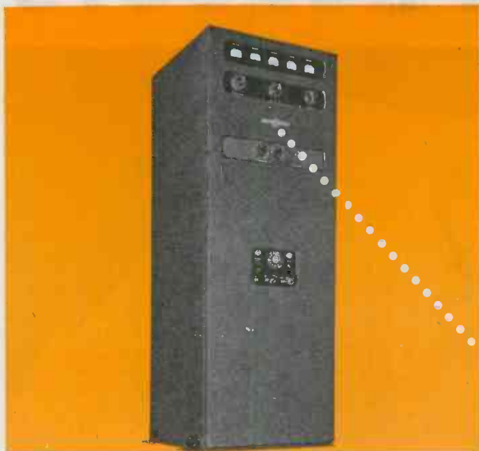
Collins 16F-9 —Nominal power output: 300 watts phone; 500 watts CW. Frequency range: 2 to 18 mc. Ten quick-shift frequencies.
