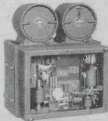
Automatic oscillograph, Type PM-13. Starts recording one-quarter cycle after disturbance occurs
